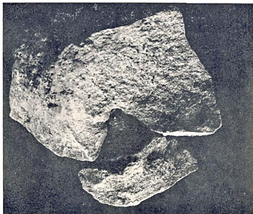
ACTUAL PHOTOGRAPH SHOWING SINGLE CONE IN CUP, AS FOUND.
